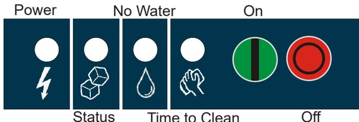
Note: If the De-Scale & Sanitize light is ON, following the cleaning process will clear the light for another cleaning time interval.
