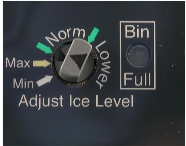
Rotate the adjustment post to the desired ice level.
